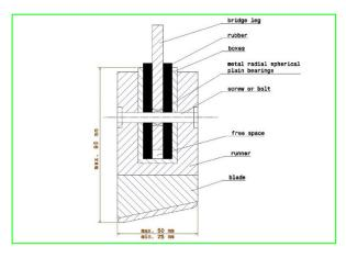
• The dimensions of the runner plus steel must not exceed 50 mm in width and 95 mm in height.
